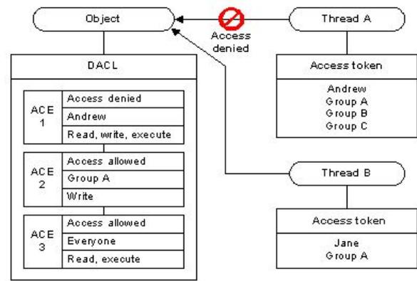
Figure 2: Example of Access Checks in Windows [4]
