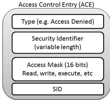
Figure 1: Access Control Entries in Windows NT
