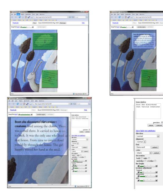
Figure 13. Transcription/Verification Interface. (top-left) blocks overview; (top-right) blocks editing view; (bottom-left) editing view close up; (bottom-right) font/layout panel close up.
