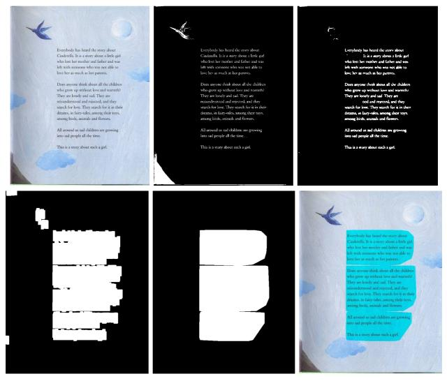
Figure 10. Steps of automatic image processing (left-to-right, top-to-bottom). (1) Input image; (2) Color thresholding; (3) Connected component analysis; (4) Dilation; (5) Text block formation; (6) Result.
