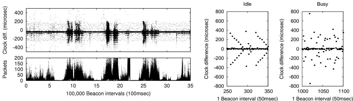
**Fig. 6.** Difference in monitor timestamps and beacon timestamps for the Sigcomm’04 “chi” trace (top left), with the load shown (bottom left). A controlled experiment with 50msec beacon intervals without load (middle) and with (right).
