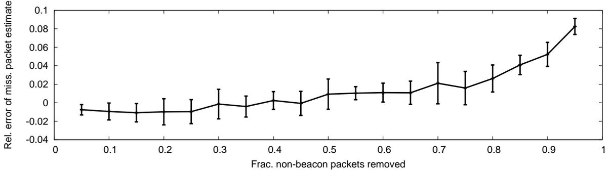
**Fig. 2.** Validation of our missing packets estimation. Starting with a high-quality trace (the Portland State University ug trace [13]), we remove non-beacon packets uniformly at random. Error bars represent 95% confidence intervals.
