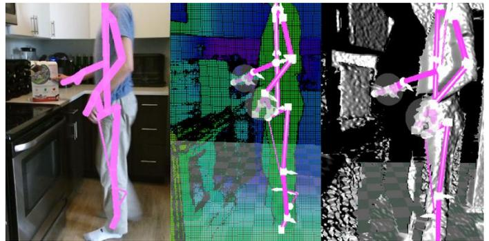
**Figure A:** In the above image, a human is reaching for a cereal box, but due to the camera angle and distance, it is difficult for the system to make an accurate prediction about the cereal box, until it is brought into a better view as shown in **Figure B**.
