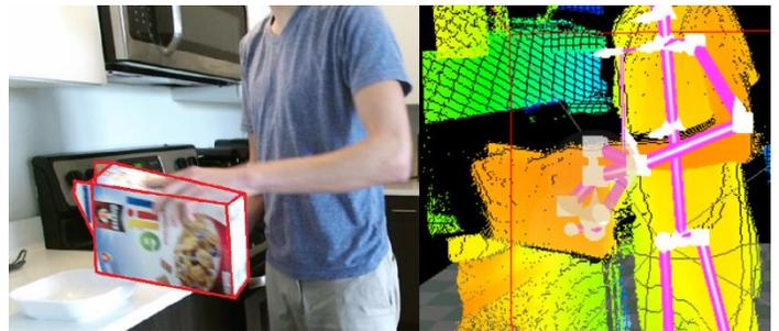
**Figure B:** Left shows a much clearer RGB image that provides much better views for texture-based recognition. Right shows depth point cloud which is much more accurate from this view.
